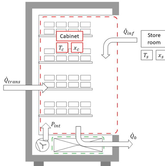
**Figure 1** Principal overview of the heat flows in a display cabinet
