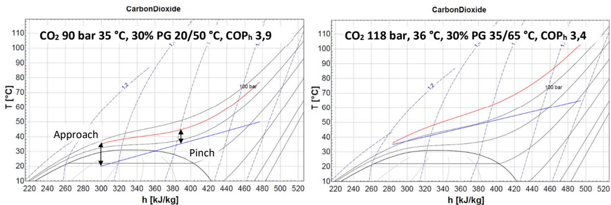
Figure 2: Gascooler temperatures in h-T diagram
