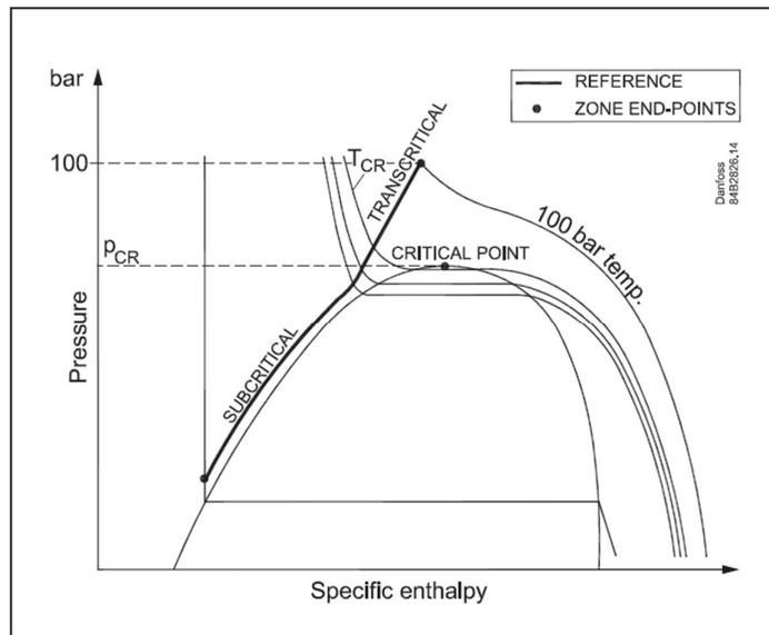
Figure 1: The reference curve for controlling the high pressure.
