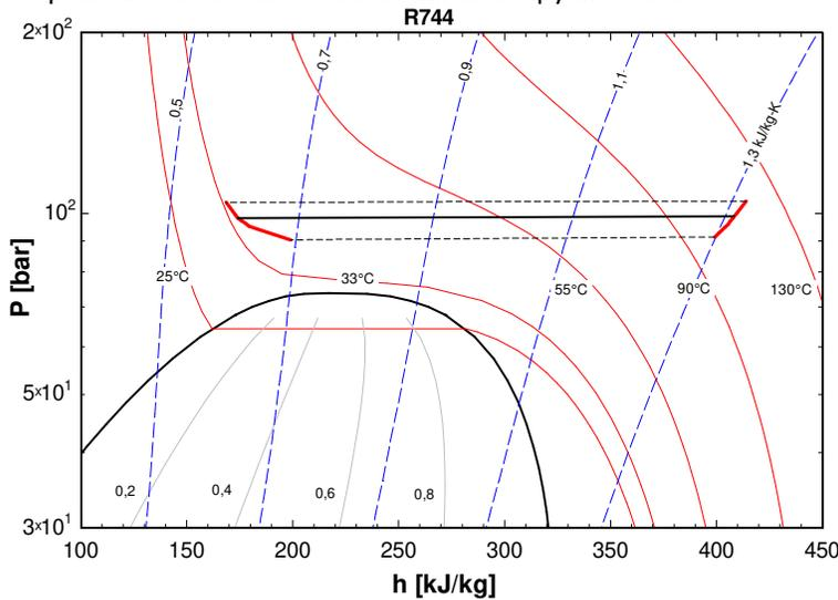
Figure 7: Diagram representing the “33 1,0 1,00” curve in the h-log(P) diagram
