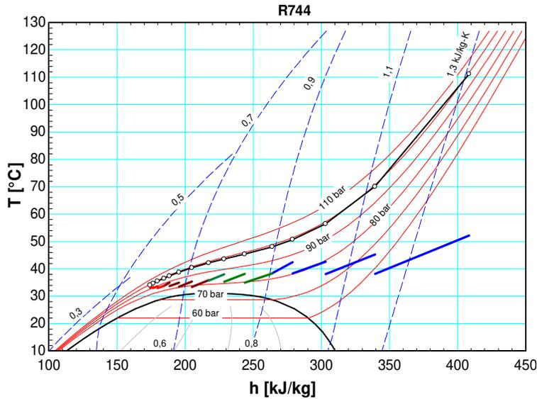
Figure 6: Diagram showing one gascooler circuit in h-log(T) diagram at 99 bar inlet pressure and 1,1 K approach
