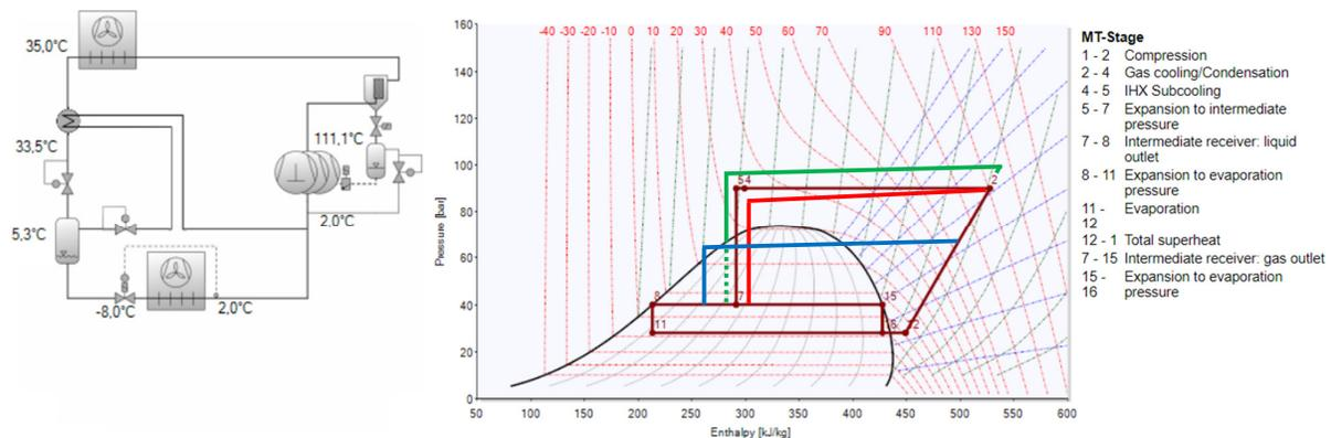
**Figure 3: System layout and representation in h-log(P) diagram**
