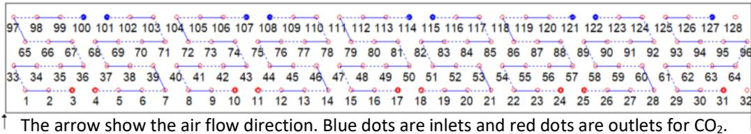
Figure 4: Configuration of the 9 circuits in the modelled gascooler
