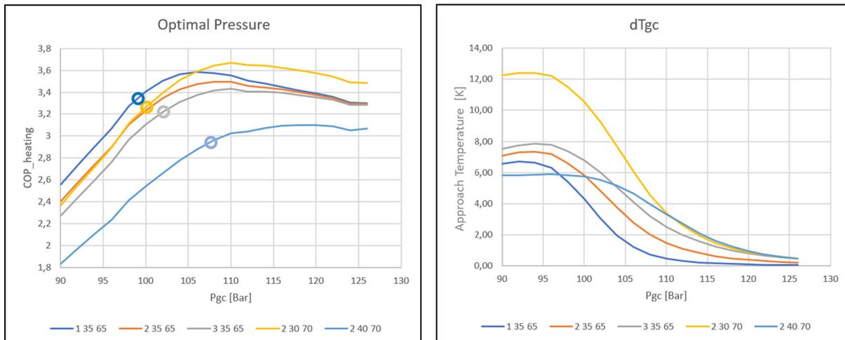
Figure 8: Optimal pressure and associated temperatures for a gascooler executed as a plate heat exchanger for heat recovery
